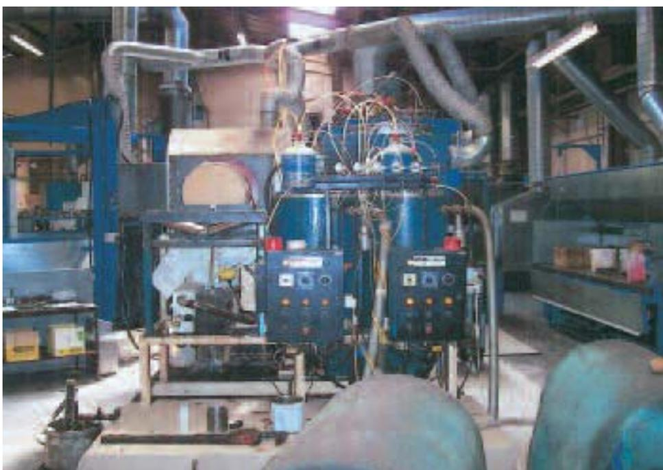
5.59 The venting area(s) should be extracted or the surrounding atmosphere will become contaminated with vapour. Two companies have installed LEV above the vent with ducting leading to the outside of the building. Any released vapour is passed through a carbon filter before release to the outside.
