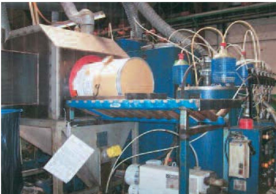
4.18 The released MbOCA pellets from the hopper and glove box (see Photo 3) are fed into the reactor vessel/dispensing machine by vacuum transfer or by gravity feed and mixed with resin, various colour pigments and catalysts. The quantity of material entering the reactor vessel is pre-set to produce the correct formulation for the required polymer.
