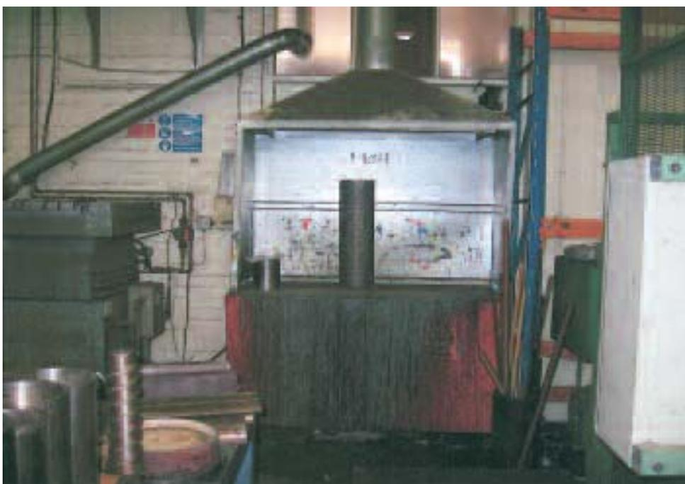
4.9 Within an LEV system the MbOCA in the container is weighed to a specified amount, the container is placed on a hot plate and the MbOCA heated to between 98°C – 105°C. The pellets melt at about 100°C. The melted MbOCA is stored at between 90°C to 100°C in the container. There will be evolution of vapour at this temperature. Some decomposition will occur if the MbOCA is heated above 140°C.
