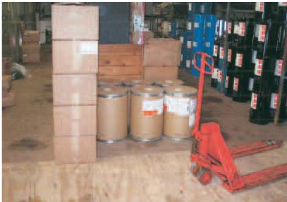
5.44 However, there is still a low risk of a keg becoming contaminated when it is lifted onto a trolley and wheeled into the work area ie hand to keg contact. A keg may be damaged by a fork-lift truck (FLT) and the MbOCA spill onto the surrounding surfaces when it is to be lifted for transfer to the work area. But this is not a common occurrence.
