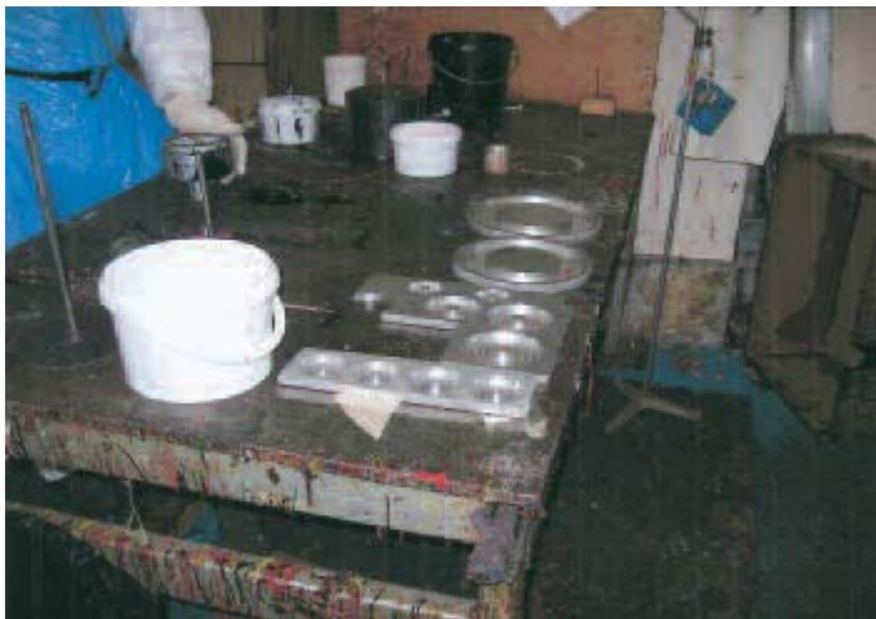
5.78 Three of the companies (K, N and O) using reactor vessels to mix the MbOCA and pre-polymer resin use unlidded containers to transport the dispensed liquid polyurethane to the casting/moulding area(s). At one of these firms (O) there was evidence of repeated splashing on the floors leading from the automated dispenser to the casting area.
