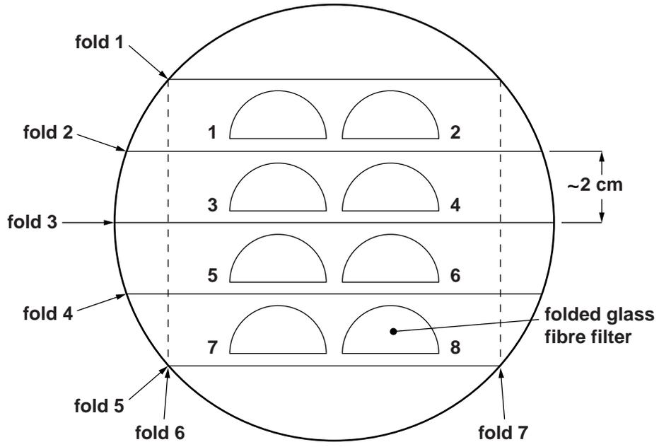
**Figure 1** Initial layout of extraction envelope
